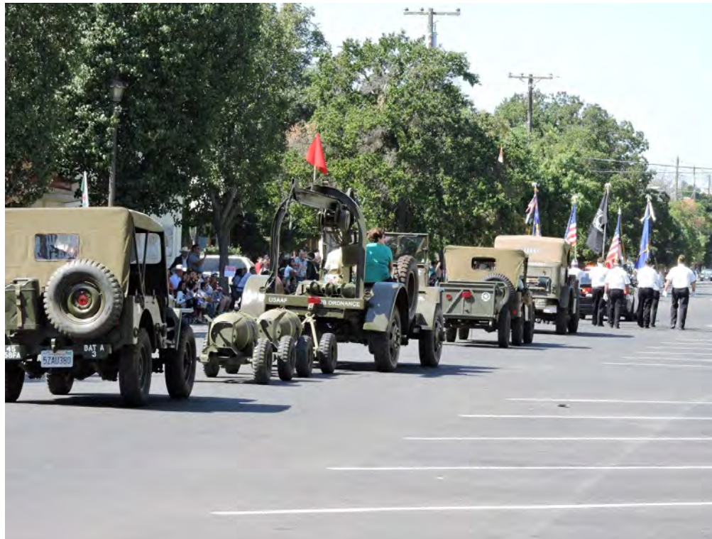
Newman Fall Festival GTBS and two M2 Bomb trailers. Dodge Half ton Command Car and two Ford GPW Jeeps Don Gomes
