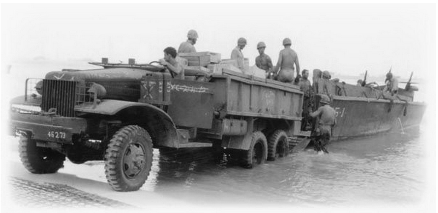
International M-5H-6 2 1/2 ton truck, Marines unload a landing craft full of supplies on the beach USMC
