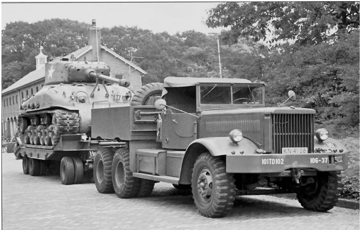
Top: Lady Marines prep a B-25 for ferrying Bottom: Diamond T 981 12 ton prime mover M20 moving a M4A3 Sherman
