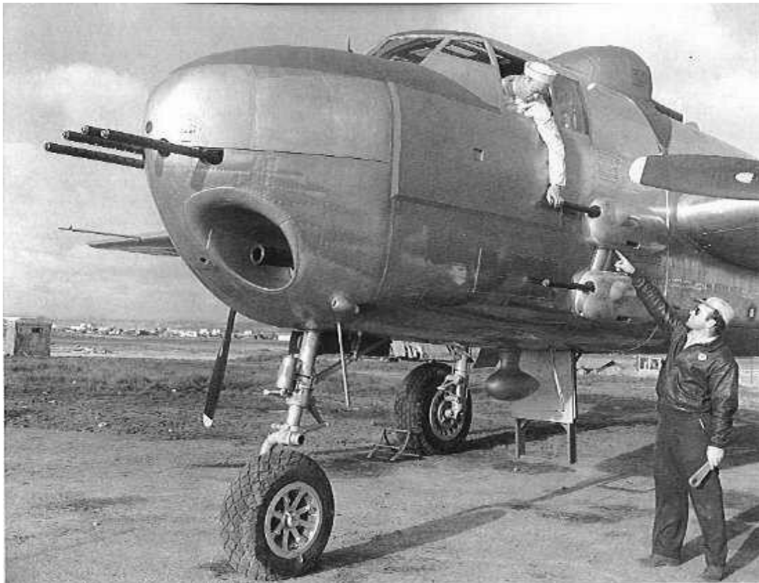
B-25G (PBJ-1G) Mitchell bombers equipped with a 75mm M4 cannon
