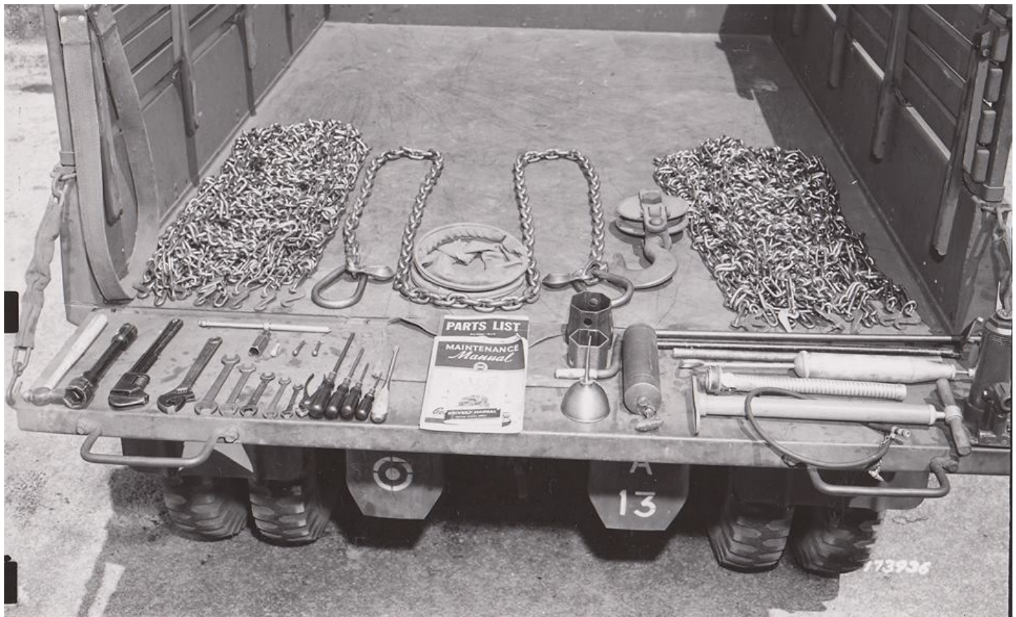
GMC, CCKW, tools and kit laid out for inspection on tailgate. Notice the two different size wheel bearing nut sockets. ED.
