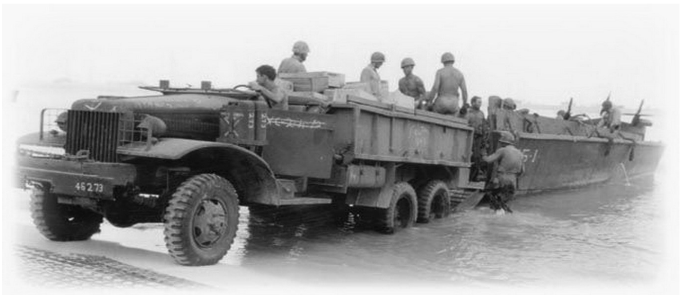
International M-5H-6 6x6 cargo truck on Island X unloading a landing craft.
