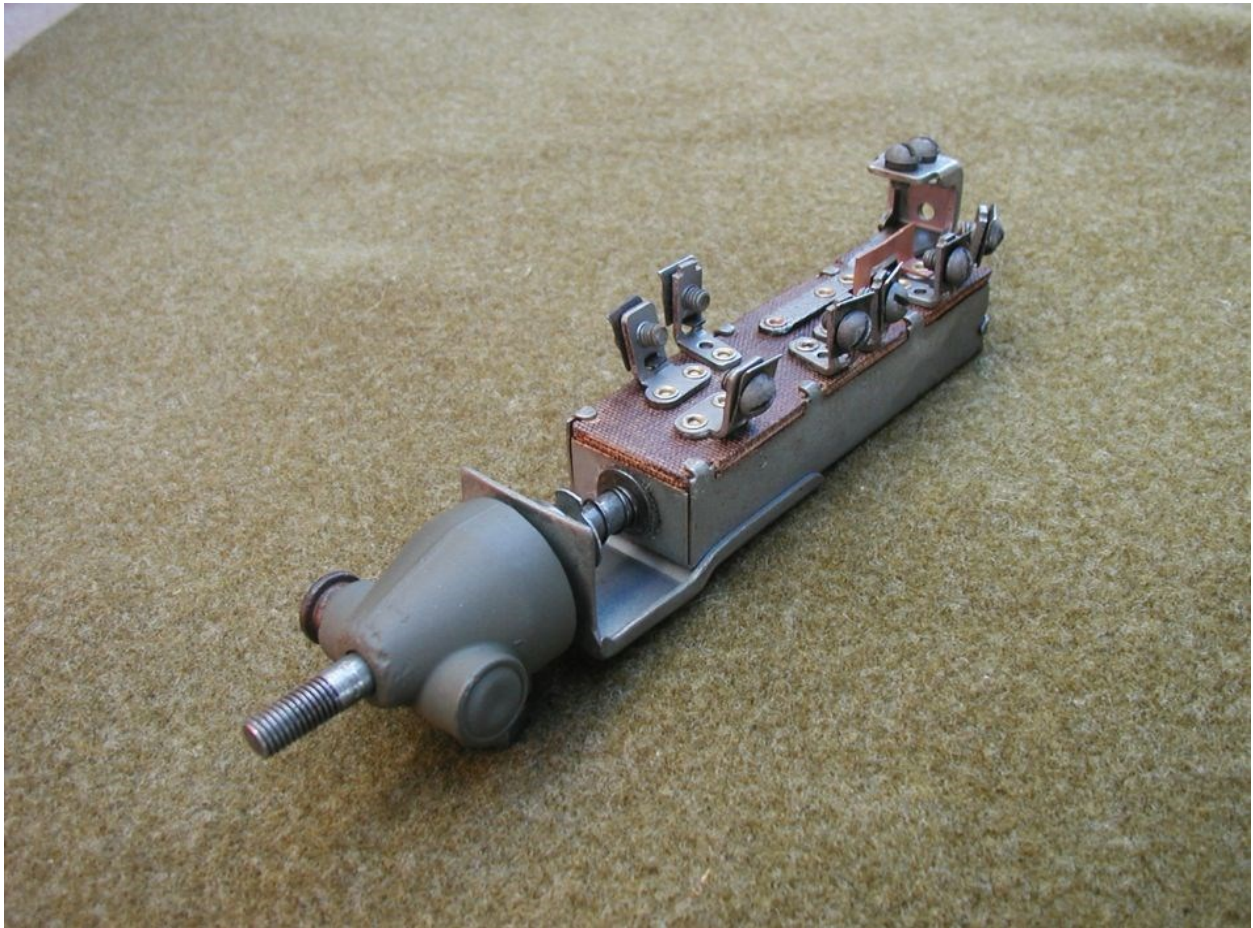
Dave Porter's Removed and Reconditioned light switch from his GTB
