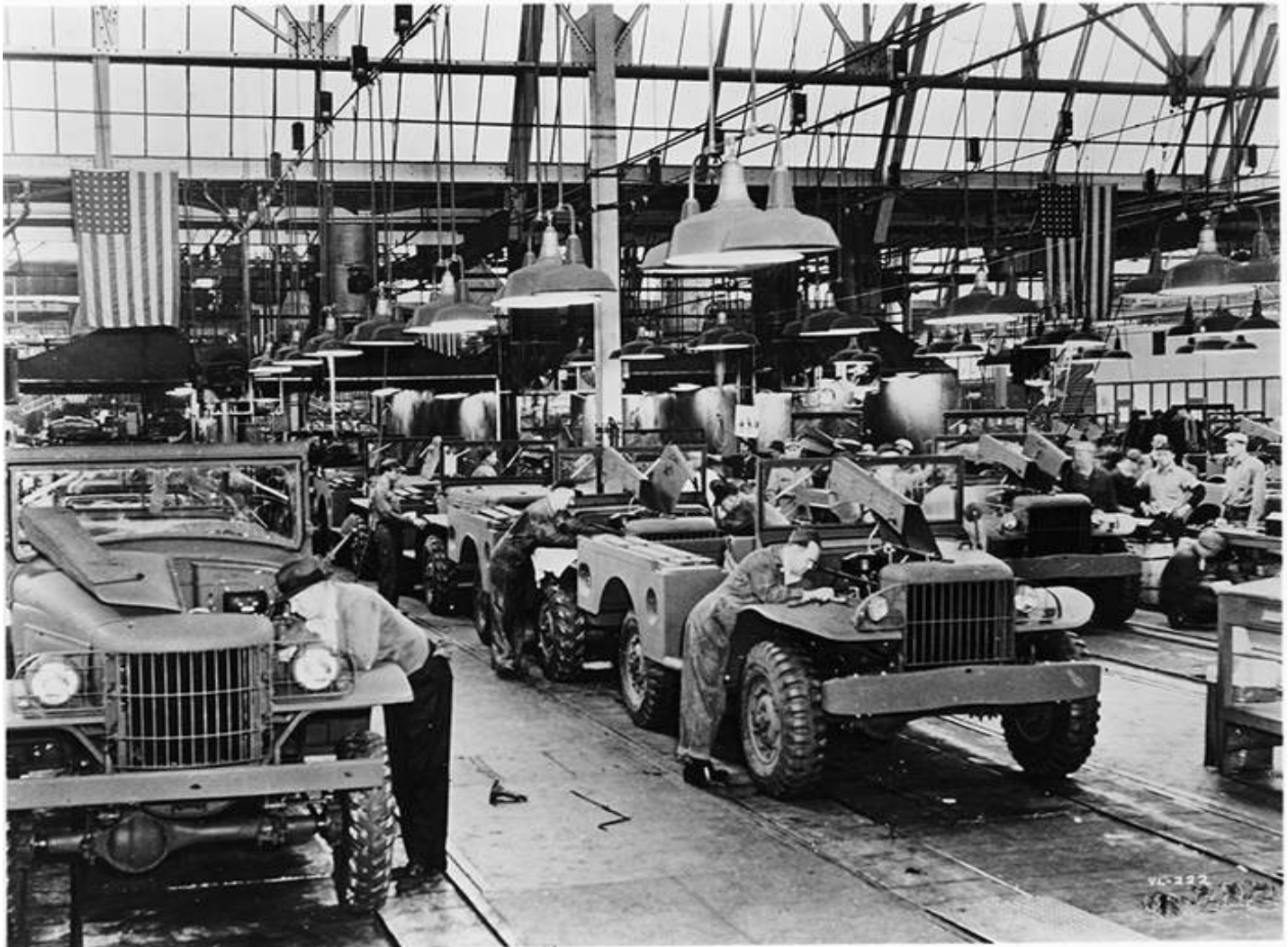
Early Dodge WC-51 3/4 ton's on the Mound Road assembly lines next to last of 1/2 ton WCs.
