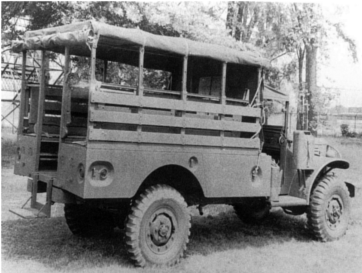
1945 Dodge 3/4 ton KD-64 Command version. Towards the end of the war these trucks were built to replace the WC54 Ambulance . They also replaced the Command Car and Carry All. US Army
